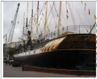
The SS Great Britain was launched in Bristol in 1843. Isambard Kingdom Brunel, conceived the groundbreaking combination of a screw propeller, an iron hull, and a massive steam engine. She was immediately successful - on her maiden voyage across the Atlantic the SS Great Britain easily broke the previous speed record.
